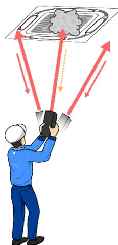
Inspection using this detector
