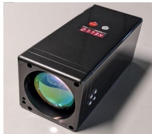
Prototype model of a portable R32 detector
