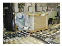
3. Pre-delivery inspection When the product is completed and packed, a refrigerant detector is once again used to ensure no refrigerant has leaked.
