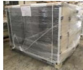
This improvement changed the packaging to entirely paper-based protective angle, while wood pallets were eliminated on all applicable models, which reduced the use of wood and cut wood material loss by 91 tons a year.
