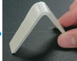
PEEK / Fluoropolymer Composite Materials (Combines high strength and flexibility)
