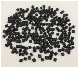
PPS/Glass Filler Composite (Achieves low cost and high functionality through our proprietary dispersion technology)
