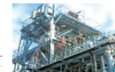
Destruction facilities for recovered fluorocarbons. After being completely broken down at a combustion destruction temperature of 1,250°C, the fluorocarbons are recycled.
