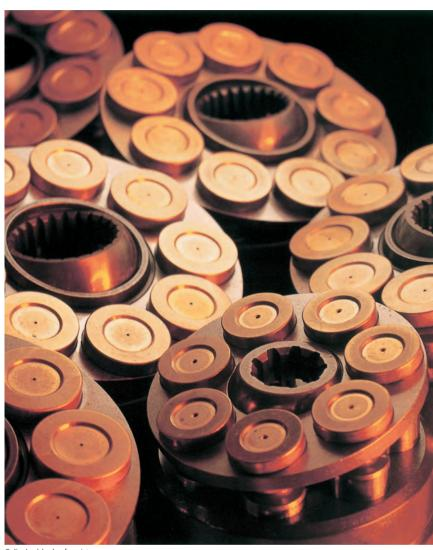
Cylinder block of a piston pump
