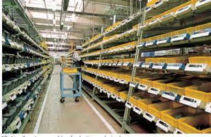
Picking" system capable of selecting a desired part from over 1,000 different types
