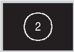
When the U5 error code appears, press
