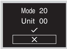
Press **←** or **→** button, move to **✗**, and then press **○** button to return to the installer menu.
