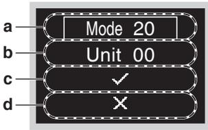
Press **+** or **-** button, to select Mode No. and press **○** button to enter the field setting menu.
