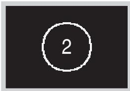
When the U5 error code appears, press
