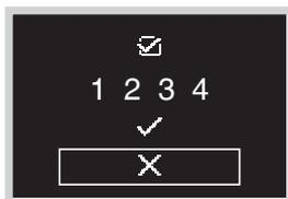
Press **-** or **+** button, move to "**X**", and then press **○** button to return to the installer menu.
