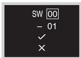
Press **+** or **-** button, scroll to the desired First code No. and then press **○** button to set the selection.
