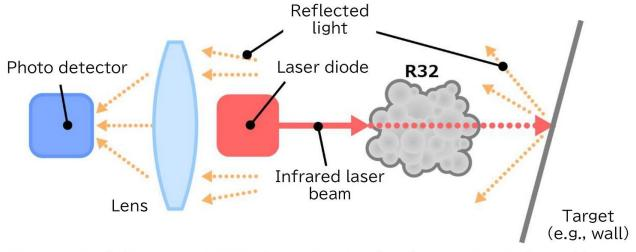
Conceptual diagram of R32 detection technology using infrared laser
