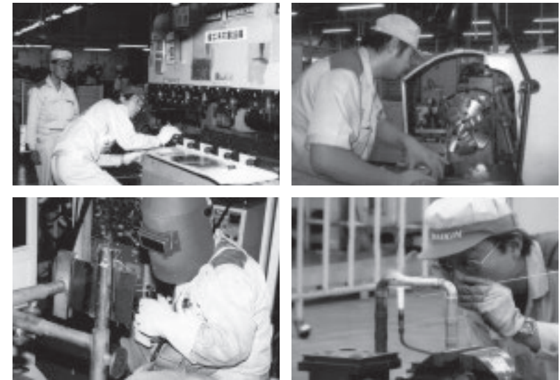
Scenes of Company-wide Technical Skills Olympics; Clockwise from upper left, Sheet metal processing, Lathe operation, Brazing, Electric welding
