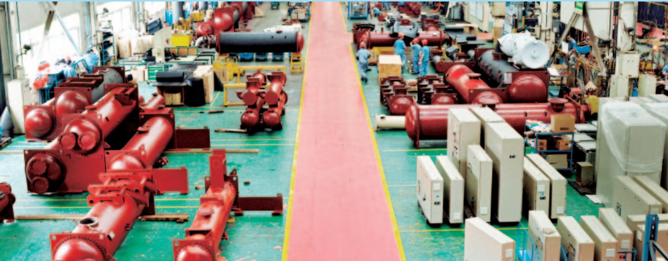
*Heat exchanger manufacturing line at McQuay Air-Conditioning & Refrigeration (Wuhan)*
