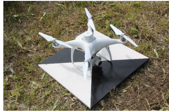
Photo 1-8. Measurement drone used for aerial photographs (July 20, 2020)
