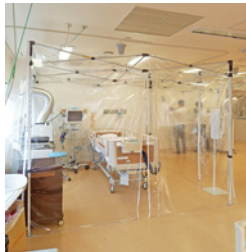
Collapsible negative pressure booth with aluminum frame
