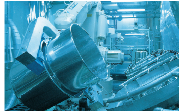
Automated fluoropolymer pellet production in the cleanroom
