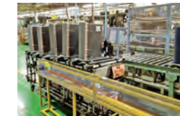
"Karakuri" is utilized for the thrust and inclination of transport vehicles to supply parts to production lines and save energy
