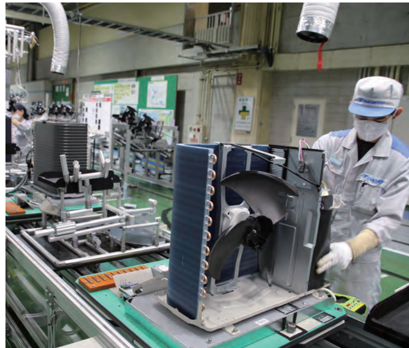
Assembly line for outdoor units
